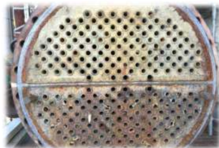
Corrosion on the Cold Inlet Fouling on the Hot Outlet
